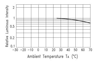
Fig.5 Luminous Intensity vs. Ambient Temperature
