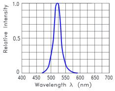
Fig.1 Relative Intensity VS. Wavelength
