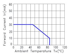
Fig.2 Forward Current Derating Curve
