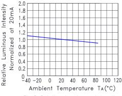
Fig.5 Relative Luminous Intensity VS. Ambient Temperature
