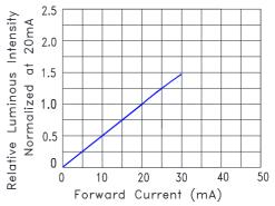
Fig.4 Relative Luminous Intensity vs. Forward Current
