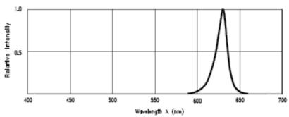
Fig.1 Relative Intensity vs. Wavelength
