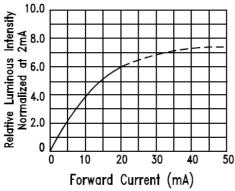
Fig.4 Relative Luminous Intensity vs. Forward Current
