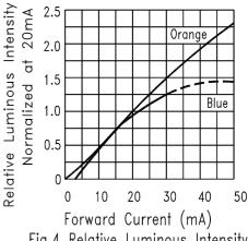
Fig.4 Relative Luminous Intensity vs. Forward Current
