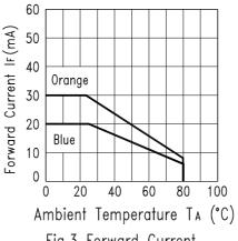
Fig.3 Forward Current Derating Curve
