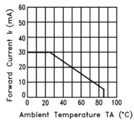
Fig.3 FORWARD CURRENT DERATING CURVE
