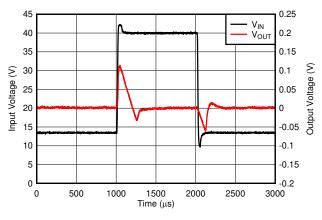
Line Transient Response (3-V/µs VIN Slew Rate)
