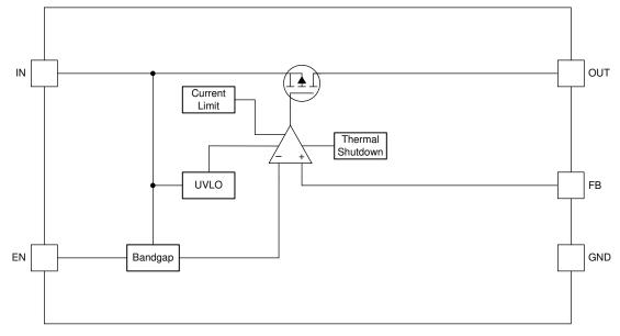
Figure 7-1. Adjustable Output Block Diagram
