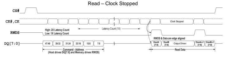
Figure 13 - Active Clock Stop during Read Transaction (DDR)
