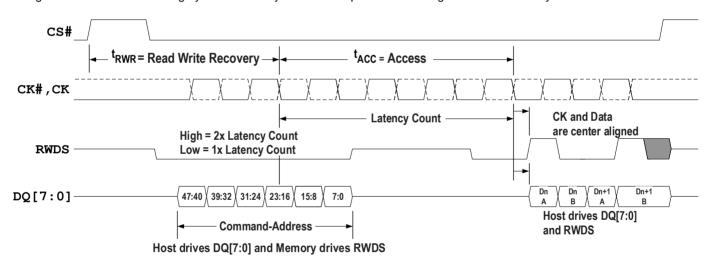
Figure 11 - Write Transaction without Additional Initial Latency
