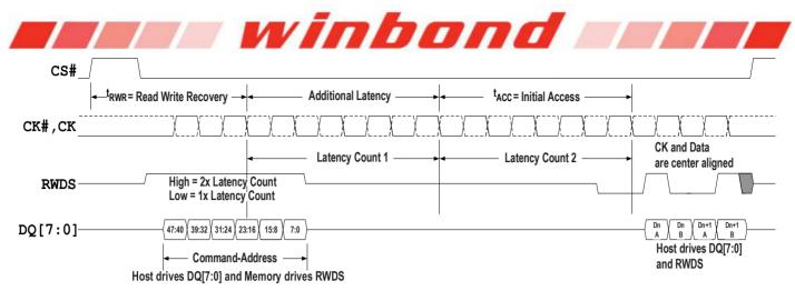
Figure 10 - Write Transaction with Additional Initial Latency
