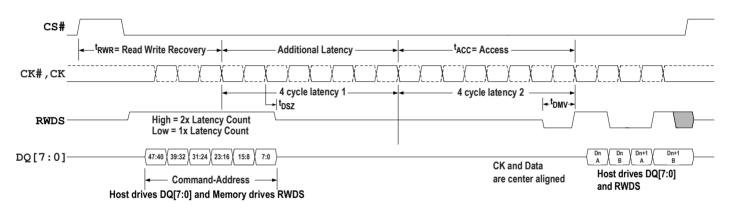
Figure 33 - Write Timing Diagram — With Additional Latency
