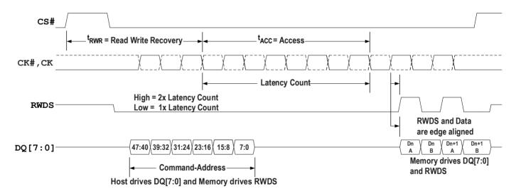
Figure 1 - Read Transaction, Single Initial Latency Count
