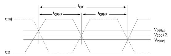
Figure 28 - Clock Characteristics
