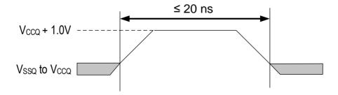
Figure 23 - Maximum Positive Overshoot Waveform
