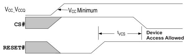
Figure 19 - Power-up with RESET# Low
