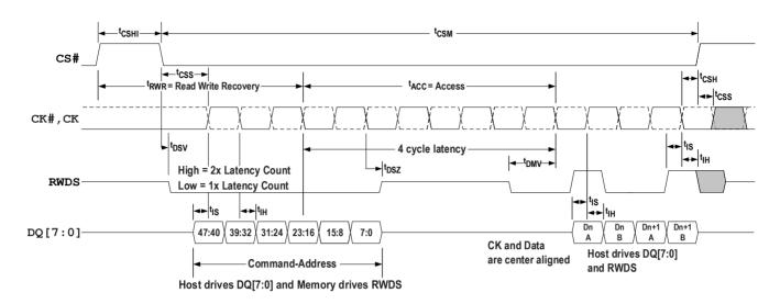
Figure 32 - Write Timing Diagram — No Additional Latency
