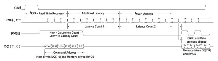
Figure 2 - Read Transaction, Additional Latency Count
