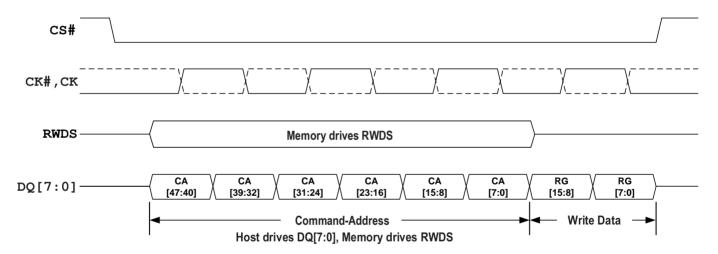
Figure 12 - Write Operation without Initial Latency
