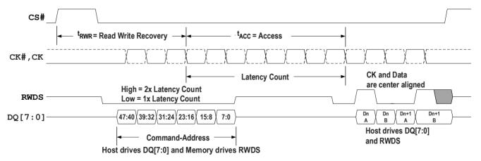
Figure3 - Write Transaction, Single Initial Latency Count
