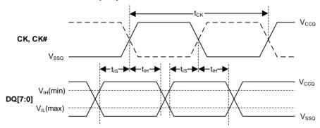
Figure 26 - DDR Input Timing Reference Levels
