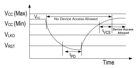
Figure 20 - Power Down or Voltage Drop
