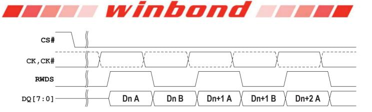
Figure 6 - Data Placement during a Read Transaction
