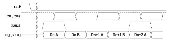
Figure 7 - Data Placement during a Write Transaction
