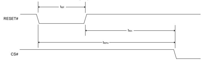
Figure 21 - Hardware Reset Timing Diagram
