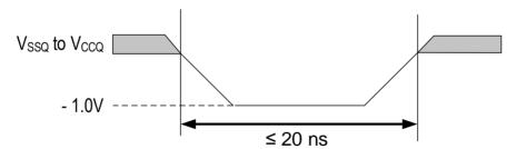
Figure 22 - Maximum Negative Overshoot Waveform
