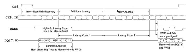
Figure 8 - Read Transaction with Additional Initial Latency
