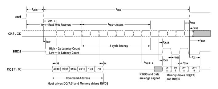
Figure 29 - Read Timing Diagram — No Additional Latency Required
