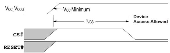
Figure 18 - Power-up with RESET# High
