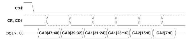
Figure 5 - Command-Address (CA) Sequence
