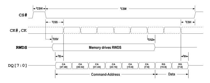
Figure 34 - Write Operation without Initial Latency (Register Write)
