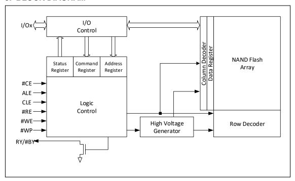
Figure 5-1 NAND Flash Memory Block Diagram
