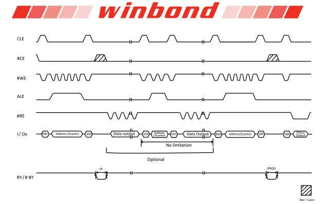
Figure 9-12 Program for copy back Operation
