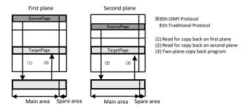
Figure 9-16 Two Plane Program for Copy Back
