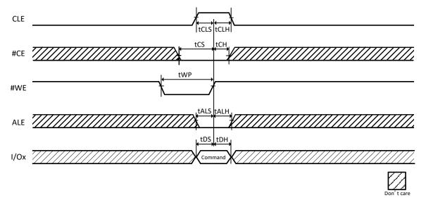
Figure 11-1 Command Latch Cycle
