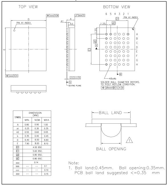
Figure 13-2 Fine-Pitch Ball Grid Array 48-Ball
