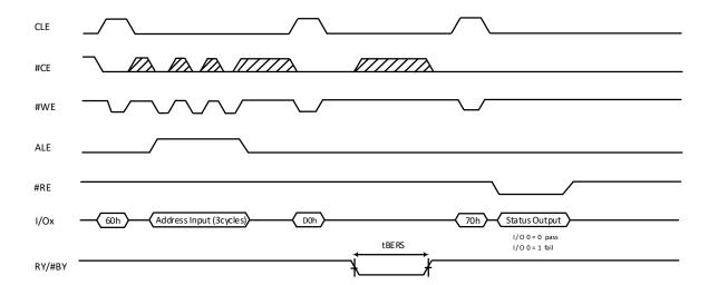
Figure 9-17 Block Erase Operation
