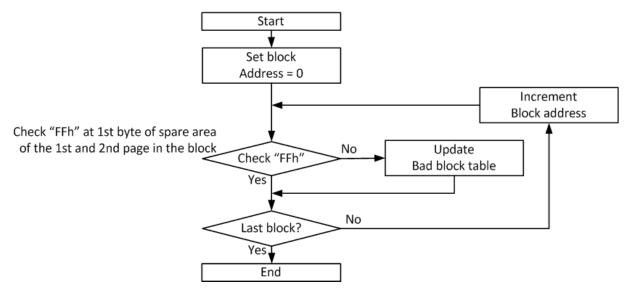
Figure 12-1 Flow Chart of Create Initial Invalid Block Table
