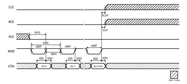
Figure 11-3 Data Latch Cycle
