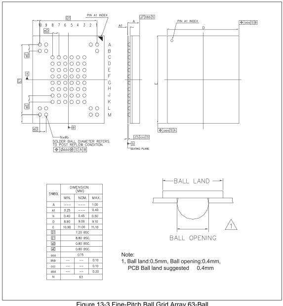
Figure 13-3 Fine-Pitch Ball Grid Array 63-Ball
