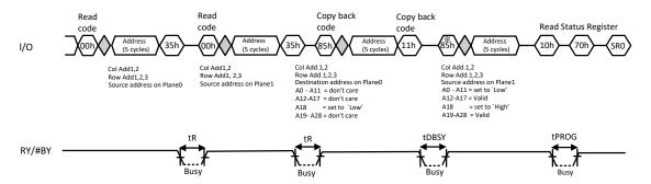
Single plane copy back read can be used to two plane operation.
