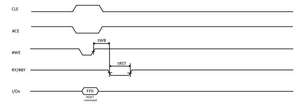
Figure 9-19 Reset Operation
