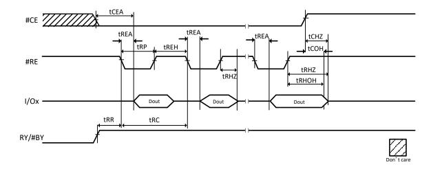
Figure 11-4 Serial Access Cycle after Read
