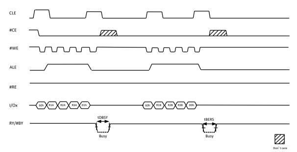
Figure 9-18 Two Plane Block Erase Operation
