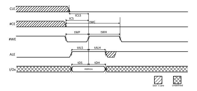
Figure 11-2 Address Latch Cycle
