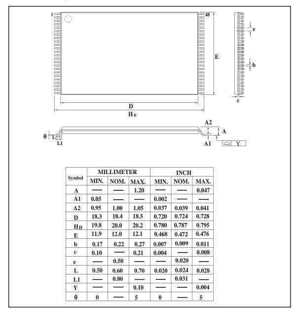
Figure 13-1 TSOP 48-PIN 12X20mm
