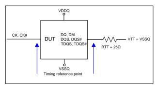
Figure 98 – ODT Timing Reference Load
