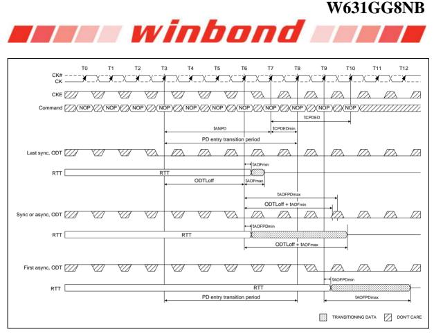
Figure 83 – Synchronous to asynchronous transition during Precharge Power Down (with DLL frozen) entry (AL = 0; CWL = 5; tANPD = WL - 1 = 4)
