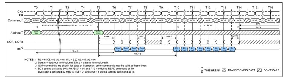
Figure 36 – READ (BC4) to WRITE (BL8) OTF
