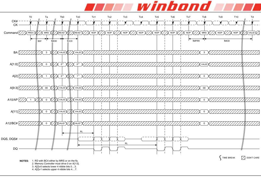
Figure 19 – MPR Readout pre-defined pattern, BC4, lower nibble then upper nibble
