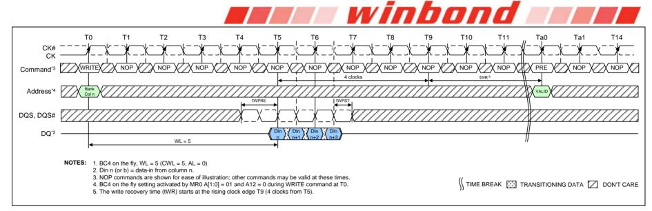
Figure 47 – WRITE (BC4) OTF to PRECHARGE Operation
