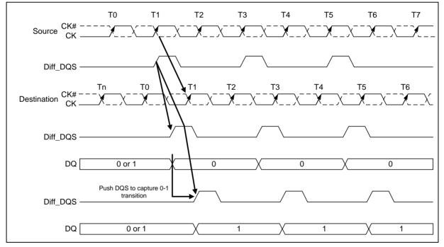
Figure 13 – Write Leveling Concept
