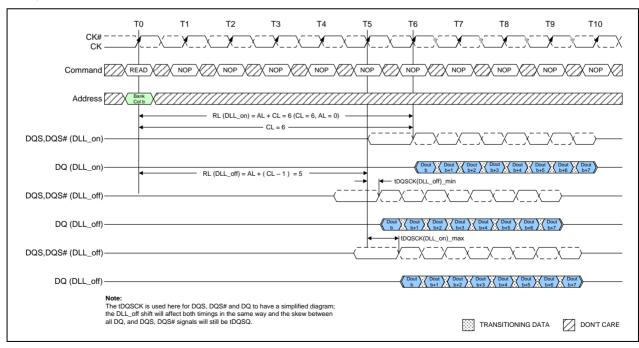
Figure 9 – DLL-off mode READ Timing Operation
