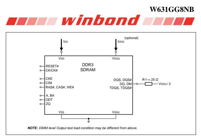
Figure 105 – Measurement Setup and Test Load for IDD and IDDQ (optional) Measurements
