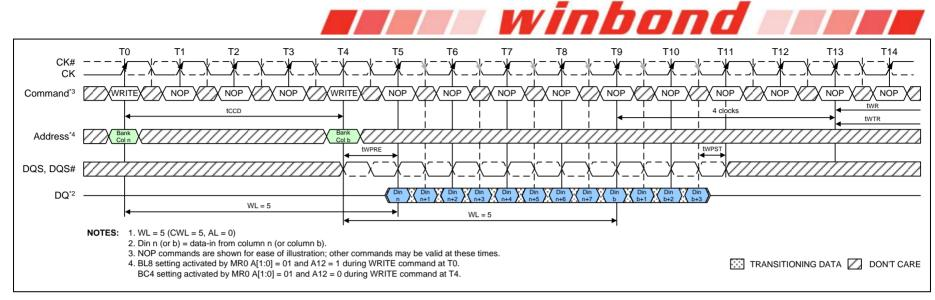
Figure 53 – WRITE (BL8) to WRITE (BC4) OTF
