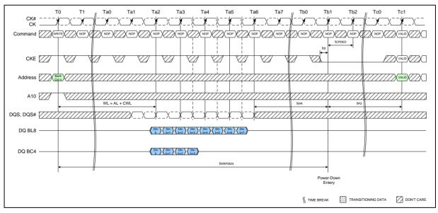
Figure 62 – Power-Down Entry after Write
