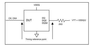
Figure 88 – Reference Load for AC Timings and Output Slew Rates
