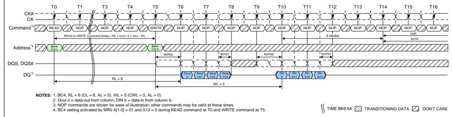
Figure 33 – READ (BC4) to WRITE (BC4) OTF
