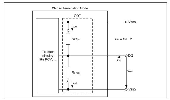
Figure 97 – On-Die Termination: Definition of Voltages and Currents
