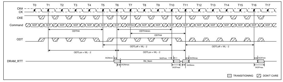
Figure 75 – Synchronous ODT (BL = 4, WL = 7)
