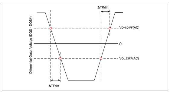
Figure 95 – Differential Output Slew Rate Definition
