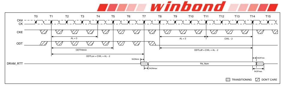
Figure 74 – Synchronous ODT Timing (AL = 3; CWL = 5; ODTLon = AL + CWL - 2 = 6; ODTLoff = AL + CWL - 2 = 6)
