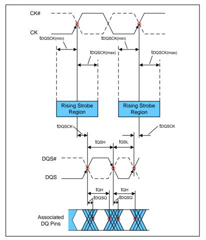
Figure 23 – READ Timing Definition
