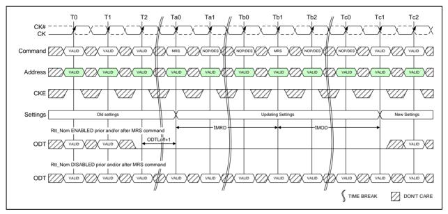
Figure 3 – tMRD Timing
