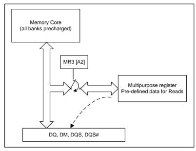
Figure 16 – MPR Block Diagram
