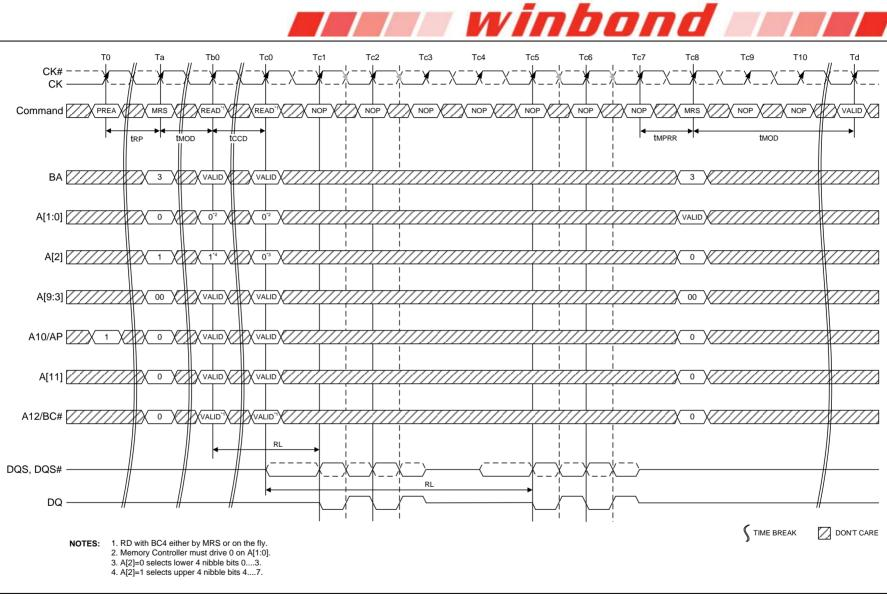
Figure 20 – MPR Readout of pre-defined pattern, BC4, upper nibble then lower nibble
