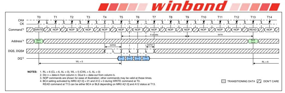
Figure 51 – WRITE (BC4) to READ (BC4/BL8) OTF
