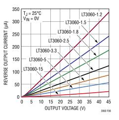
Figure 8. LT3060-1.2/-1.5/-1.8/-2.5/-3.3/-5/-15 Reverse Output Current
