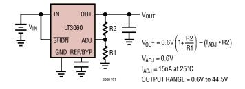
Figure 1. Adjustable Operation
