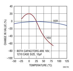
Figure 5. Ceramic Capacitor Temperature Characteristics
