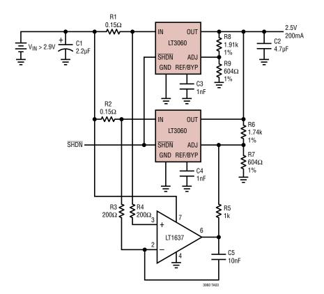
Paralleling of Regulators for Higher Output Current
