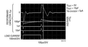
Figure 3. Transient Response vs Feedforward Capacitor
