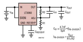
Figure 2. Feedforward Capacitor for Fast Transient Response
