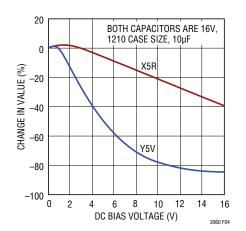
Figure 4. Ceramic Capacitor DC Bias Characteristics
