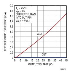
Figure 7. LT3060 Reverse Output Current
